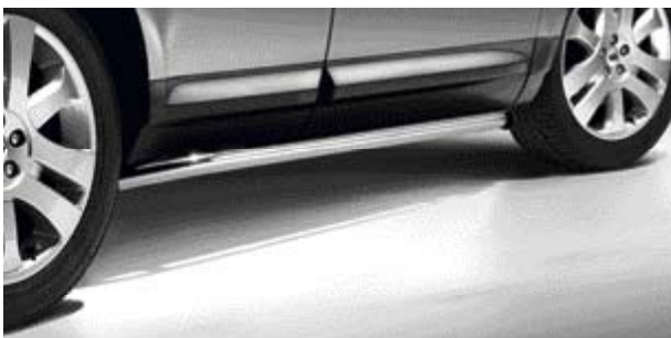
Side Protection Tube Stainless Steel LR003318
