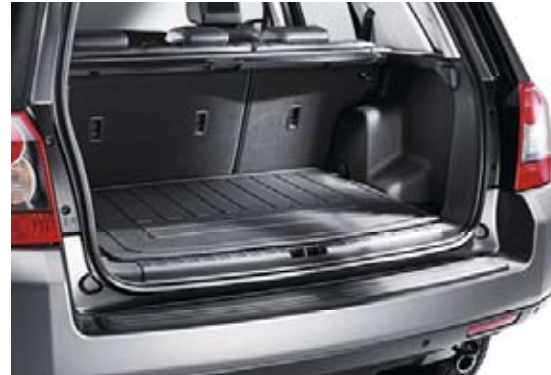
Loadspace Rubber Mat VPLFS0001 Waterproof with retaining lip and non-slip surface.
