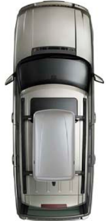
Luggage Box* VPLDR0003 Lockable for security. Opens from both sides. External dimensions: 1,600mm long, 960mm wide, 410mm high. Volume 450 litres. Load capacity 60kg.
