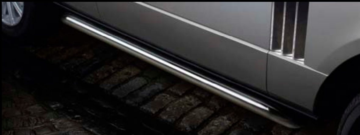
Side Protection Tubes - Stainless Steel VUB001230 Can be fitted with or without Front Mudflaps.
