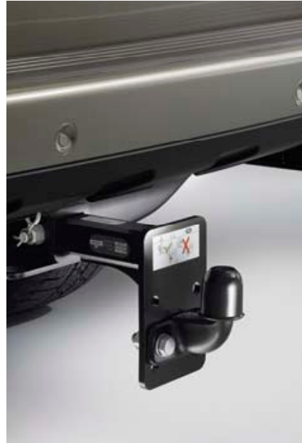
Multi-Height Tow Bar VUB000720 Offers three different towing height options. Lowest tow ball position 360mm from ground. 3,500kg trailer load capacity (250kg trailer nose load).
