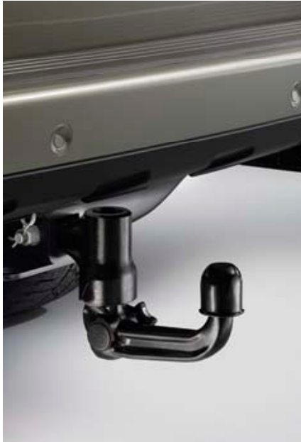
Quick Release Tow Bar VUB000730 Easily removed. Lockable for security. 3,500kg trailer load capacity (250kg trailer nose load).
